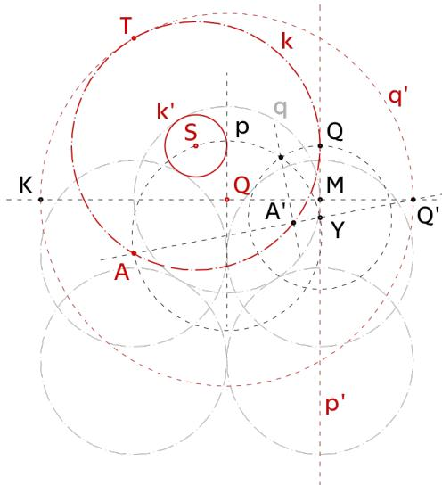
Fig. 2: Problem of Apollonius: solution of the case ‘CCC’
