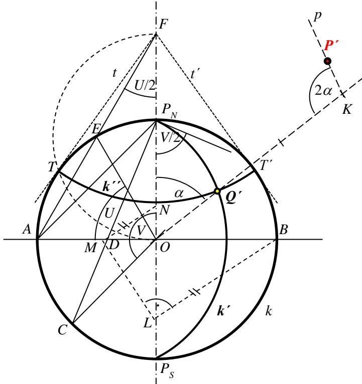
Fig. 10: The construction of a point in August's conformal epicycloidal projection [5]
