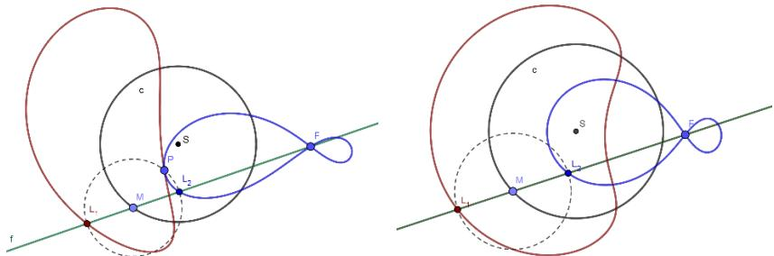
Fig. 2: Generalised strophoid and conchoid for a given circle  $c$ .
