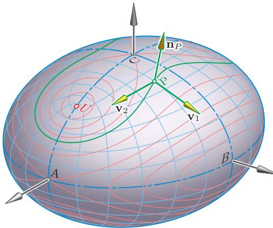
Fig. 1: Curvature lines (blue), curves of constant ratio of principal curvatures  $\kappa_1 : \kappa_2$  (red), and direction vectors  $\mathbf{v}_1, \mathbf{v}_2$  of the principal curvature tangents at  $P$ .
