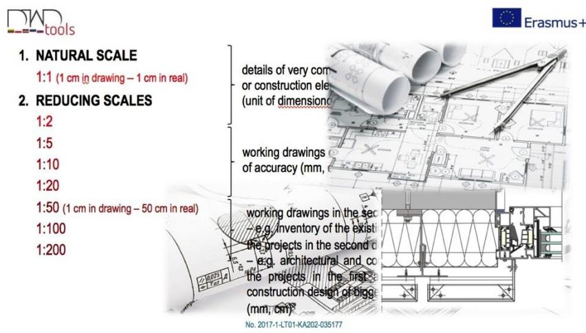
Fig. 2: The graphic layout used for dictionary parts of teaching materials in the field of architectural-construction drawing - part 3. Scales at architectural-construction drawing and part 4. Graphic designation of the building materials
