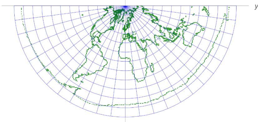
Fig. 4: World and geographic network in conical equidistant projection
