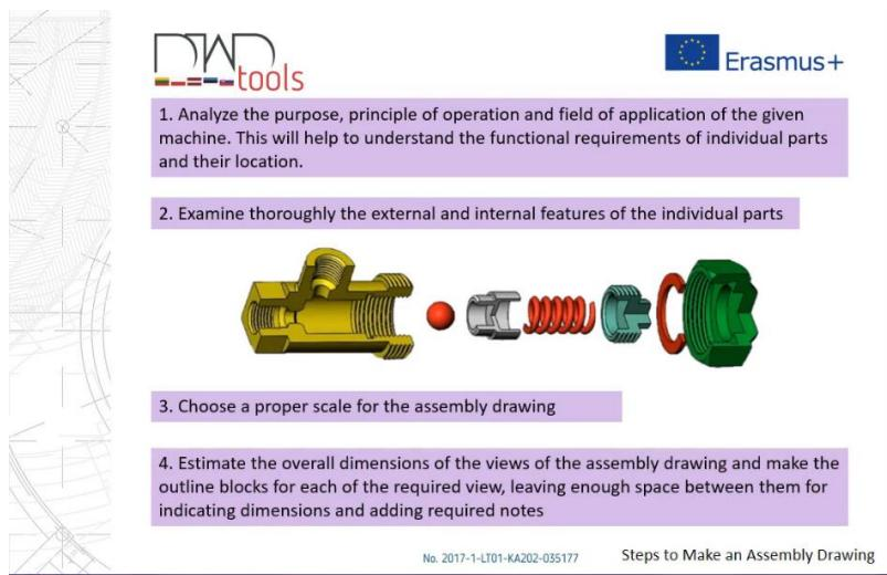
Fig. 8: Steps to make an Assembly Drawing
