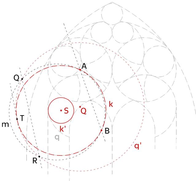
Fig. 4: Problem of Apollonius: solution of the case ‘CCC’
