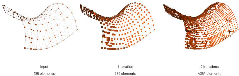
Fig. 5: The refinement on a hyperbolic paraboloid. (a) The input set with 185 elements. (b) The refined set after 1 iteration with 686 elements. (c) The refined set after 2 iterations with 4354 elements.
