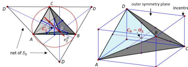
Fig. 6: Top-view and net of  $S_3 = ABCD$  (left) and axonometric view (right).
