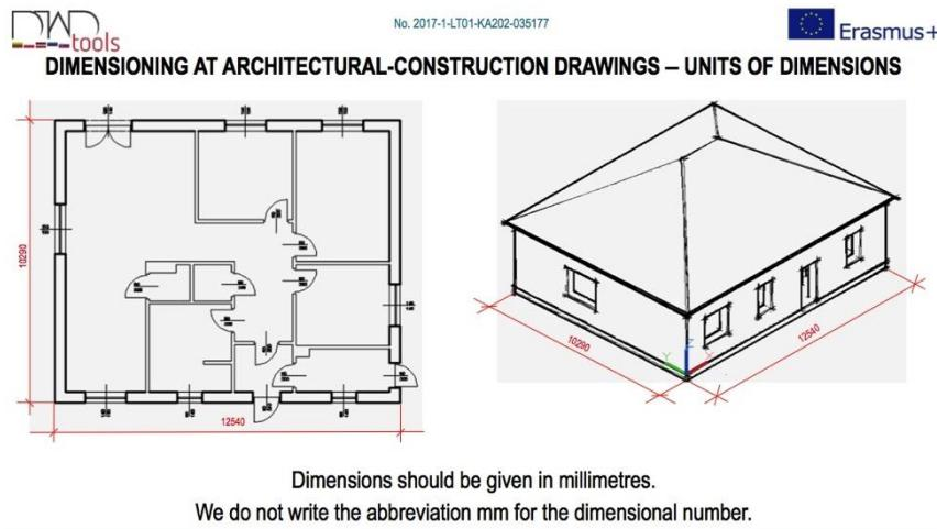
Fig. 1: The graphic layout used in three parts of teaching materials in the field of architectural-construction drawing - axonometric drawing, orthographic projection of a building object and verbal commentary discussing the presented issue.
