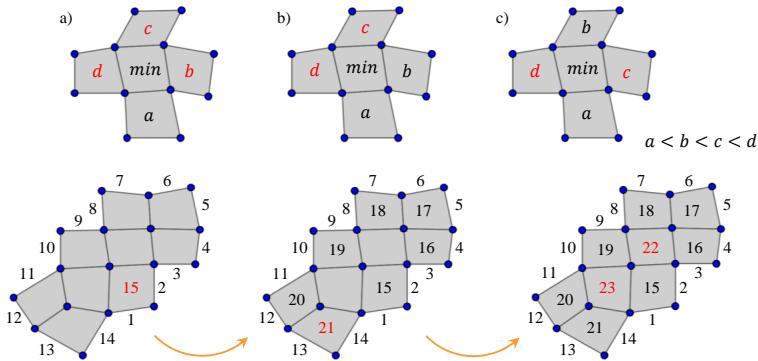
Fig. 1: Three cases (a, b, and c) of numbering of quadrilaterals in quadrilateral mesh and an example of a unique numbering of a quadrilateral mesh in three steps.
