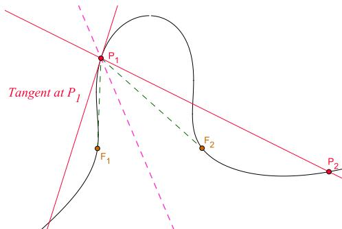
Fig. 5: Construction of a tangent at the point  $P_1$
