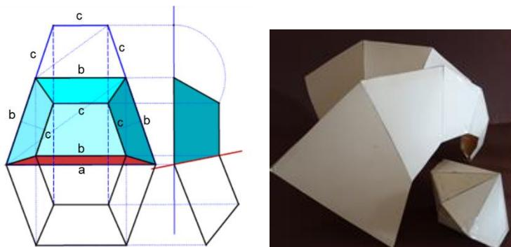
Fig. 15: A closed polyhedron with similar isosceles trapezoids as faces, (left); an infinite spiral polyhedron with quadrangular faces, (right).
