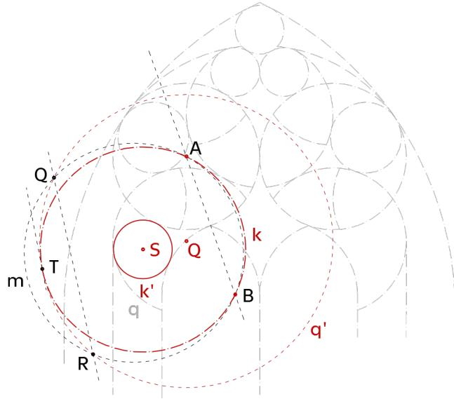
Fig. 4: Problem of Apollonius: solution of the case ‘CCC’
