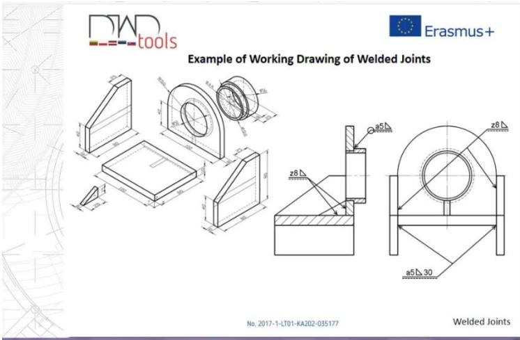
Fig. 7: Example from video Separable and permanent joints
