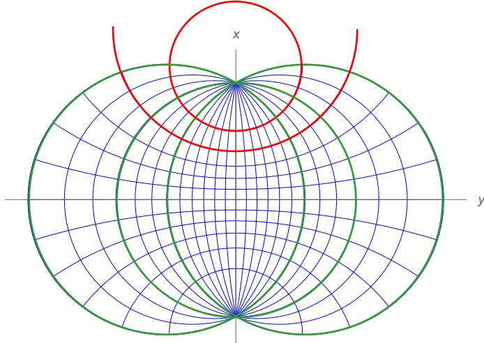
Fig. 5: Geometric properties of Lagrange's conformal projection
