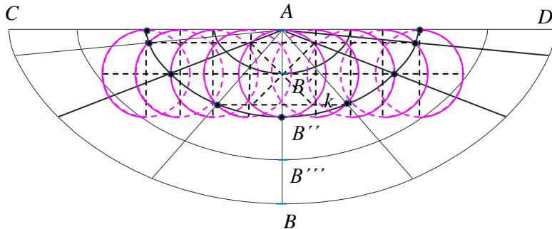
Fig. 3: Geometric construction of Jervis's projection
