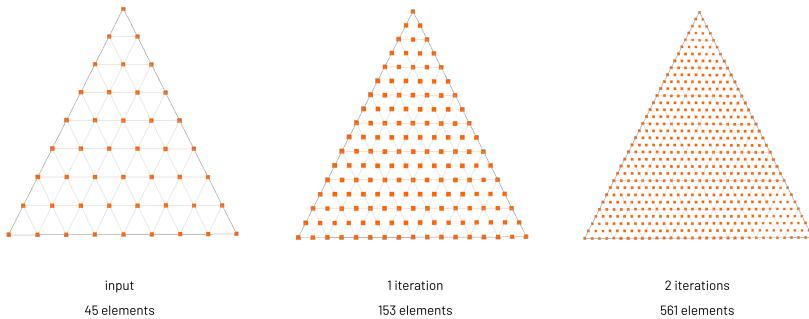
Fig. 3: The refinement on a part of a plane. (a) The input set with 45 elements. (b) The refined set after 1 iteration with 153 elements. (c) The refined set after 2 iterations with 561 elements.
