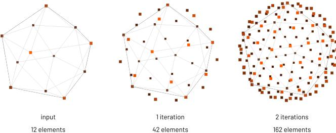
Fig. 4: The refinement on a sphere. (a) The input set with 12 elements. (b) The refined set after 1 iteration with 42 elements. (c) The refined set after 2 iterations with 162 elements.
