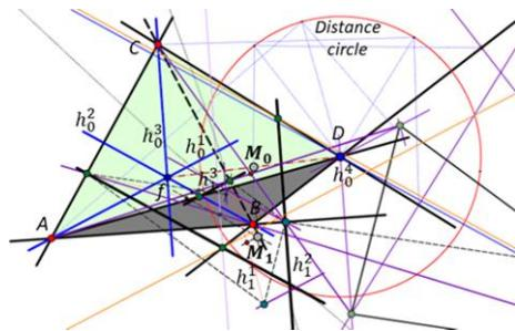
Fig. 2: Top-view of a tetrahedron with its 0- and 1-altitudes  $h_0^i$  and  $h_1^j$  as well as its Monge points  $M_0, M_1$  (general case).
