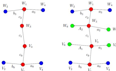
Fig. 1: Input and output of Chiyokura Kimura method
