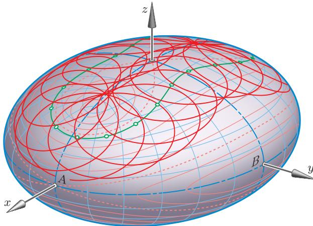
Fig. 2: Moving an ellipse on an ellipsoid.
