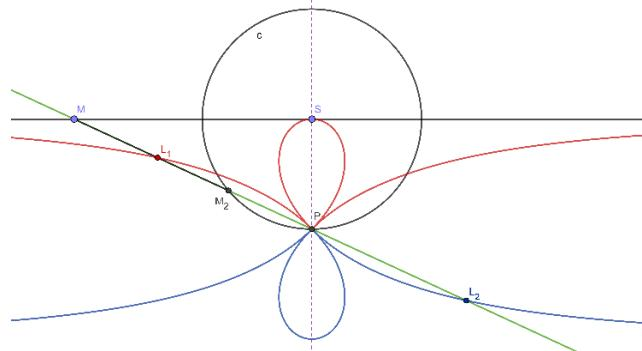
Fig. 4: Right strophoid constructed as a cissoid
