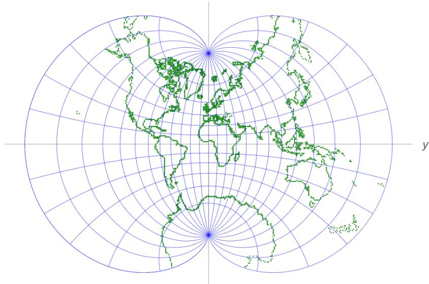
Fig. 9: Image of the geographic network in August's conformal epicycloid projection [5]
